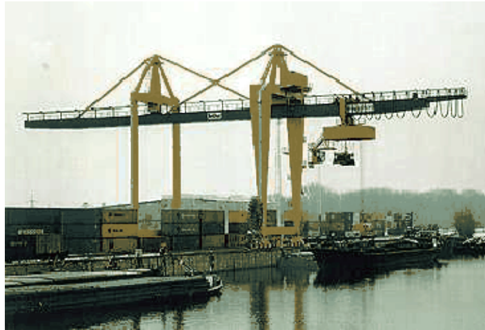
Figure 34: View of a portal-type loading crane (adapted from http://www.atp.ruhr-uni-bochum.de )
